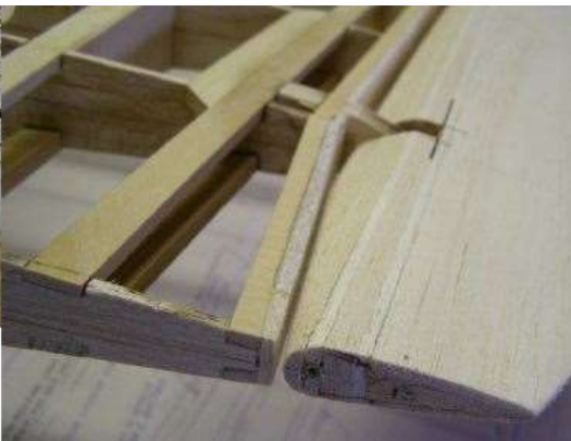
(Above) final aileron installation complete. The wing is now sheeted and made ready to be finished.
