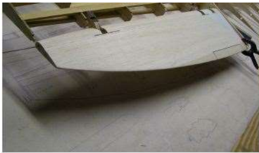
(Above) Mating aileron and hinges to main wing structure.
