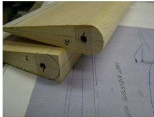
(Above) Elevator hinging assembly details, before and after sheeting and before and after shaping the leading edge.
