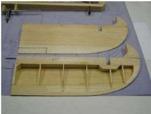
(Above) Elevator hinging assembly details, before and after sheeting and before and after shaping the leading edge.
