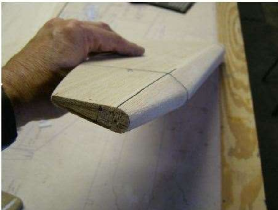
(Above) aileron tip shaped to final profile.
